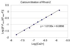
Figure 1. Example of a calcium calibration curve for Rhod-2 (Kd = 1 uM).
