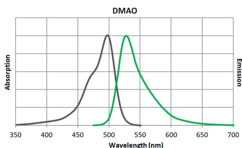
Figure 1. Normalized absorption and emission of DMAO.
