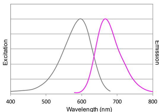
Figure 1. Normalized excitation and emission spectra of NucSpot® Far-Red in TE buffer with dsDNA.
