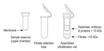
Figure 1. Ultrafiltration vial components.
