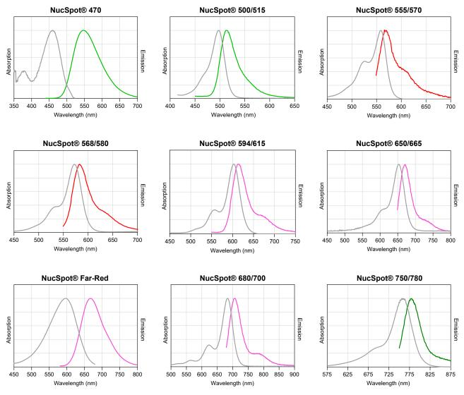
Figure 1. NucSpot® Nuclear Stains absorbance and emission spectra (with DNA).
